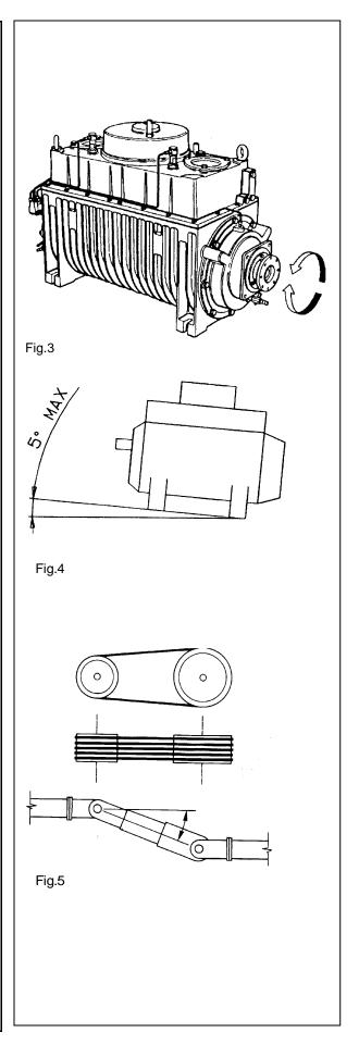
The pump pulley cannot be used as a drive for other mechanisms.
